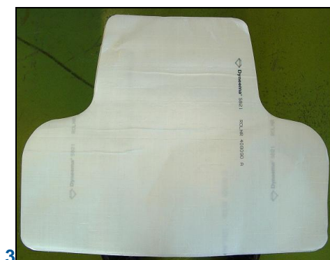
Pic 3 & 4 – Cut-out of a single sheet Dyneema® UD typically used for a vest
